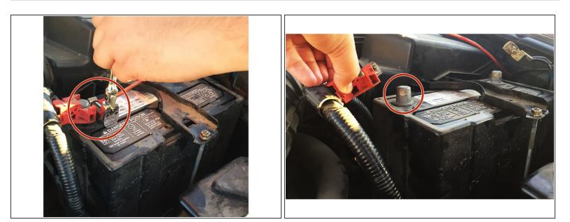
Loosen and remove the positive (Red) cable from the terminal.
