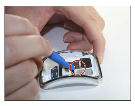
Use the plastic opening tool to gently pry upwards on the speaker's ribbon connector.
