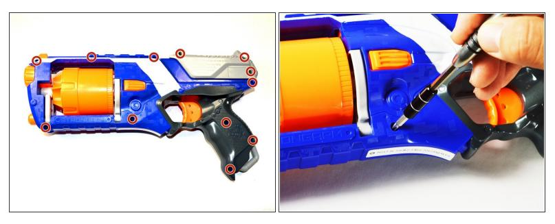
Locate the 12 Philips head screws and remove them: Head Diameter= 4.3mm, Thread Pitch= 1mm, Screw Length= 8mm
