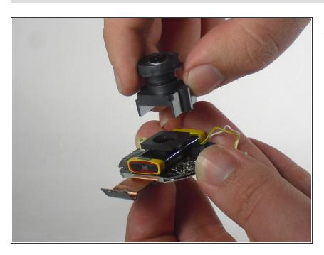
With the screws gone, lift the camera lens away from the remaining components.
