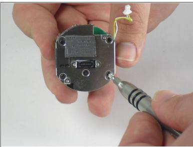
Using a Philips #0 screwdriver, remove the four 2 mm screws.
