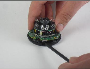
Insert a spudger tool under the micro-USB port and lift to separate the motherboard from the back case.
