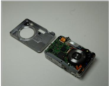
• Remove the front casing from the body of the camera.
