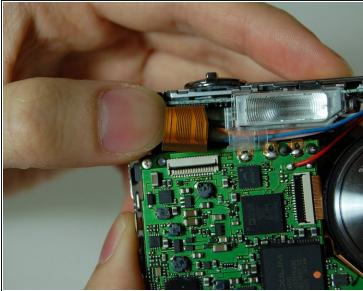
On the front of the camera, near the flash flip, there is a connector holding a ribbon. Remove the ribbon from the connector.
