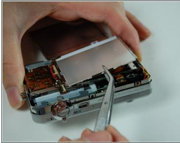
• Pry the LCD casing from the tape that is underneath it and then flip it to the opposite side to expose the contents under it.
