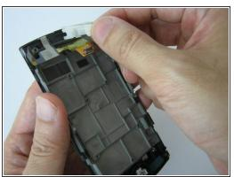
Remove the two rubber pieces from the ends of the panel.
