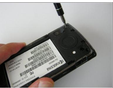
Remove the six 3.18 mm screws using a Phillips 00 screwdriver.
