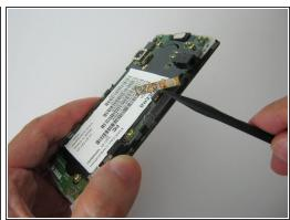
Unclip the two flex cables -- a small one located on the left side on the lower half of the motherboard, and a longer one on the right side, higher up.
