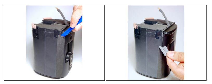
• Using a plastic opening tool, remove the grey tape from both sides of the device.
