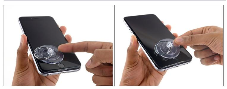
• Pull up on the small nub on the suction cup to remove it from the display.
