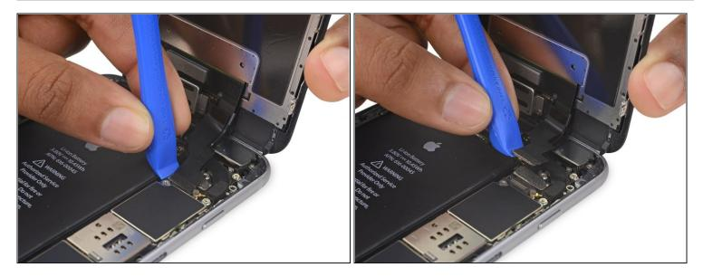
A Be careful to only pry up on the connector itself and not the socket on the logic board.
