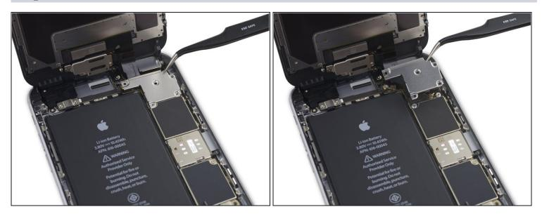
• Remove the display cable bracket.
