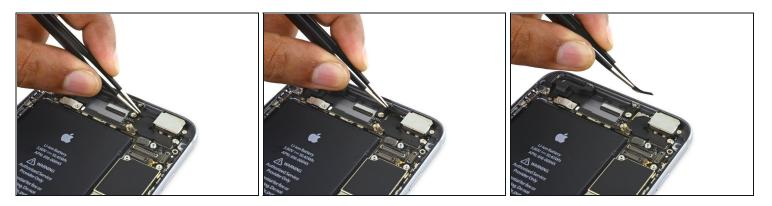
• Peel up any tape covering the iSight camera bracket screws.
