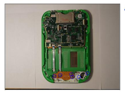
Find the screws on the bottom of the device holding down the button and speakers board.
