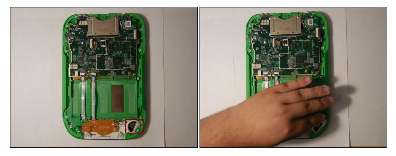
• There should be a plastic covering over the speaker, carefully pull on the opposite side from the plastic clip holding it in place.
