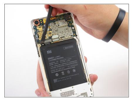
Use a nylon spudger to pry upwards to detach the ribbon that's connecting the battery to the motherboard.
