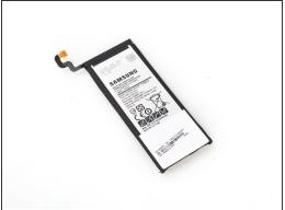
Remove battery. But it's not necessary. You also can just release battery connector from motherboard.
