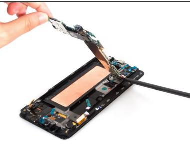
Release the USB board connector on the back and remove the motherboard from front assembly.
