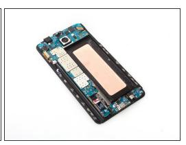
Release the connector on the board.
