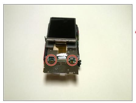
Remove the two clasp using a plastic spudger
