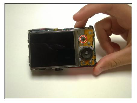
Using a Phillips #00 screwdriver, remove the PH 2mm screw located to the right of the screen, above the OK dial.
