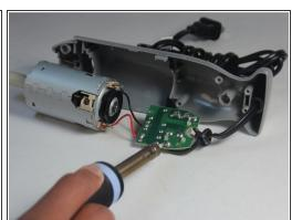
• Refer to these steps on <u>Soldering</u> to replace the electrical cord in the smart stick.
