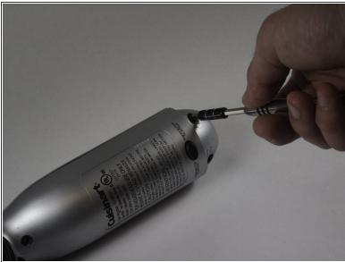
Remove three 13.3 mm Phillips PH#2 screws.
