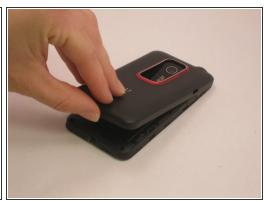
Remove the outer casing of the phone with your hands by prying and lifting at the latch.
