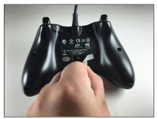
Remove the tamper seal sticker from the back of the controller.
