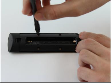
Locate the four 3.6 mm Phillips J#00 screws found under the back panel of the remote control and remove them.
