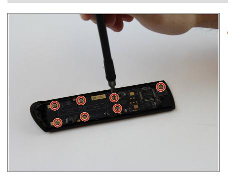
J#00 screws that connect the motherboard to the case.
