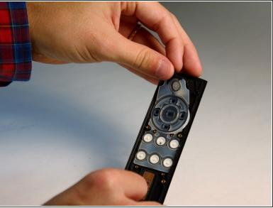
Locate the black plastic tab at the top end of the button panel, grab it with your fingers and pull back to separate the button panel from the remote control's case.
