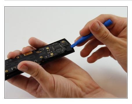
Place the plastic opening tool or your fingernail in the gap at the top end and lift the motherboard.
