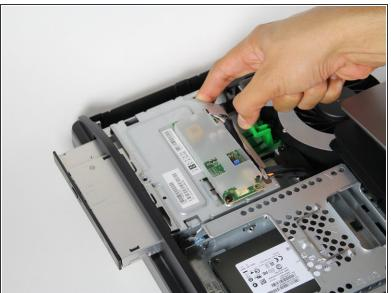
• Push the top right corner to the left, and push out the optical drive while holding up the green tab.
