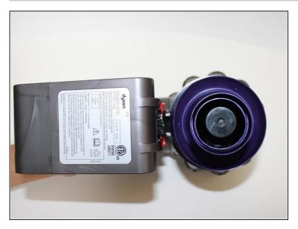
• Flip the vacuum over so that the silver cyclone part of the vacuum is now at the base.
