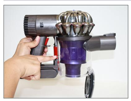
Push the red lever downward to open the clear bin. You may need to do this over a trash bin if there is debris in the clear bin.
