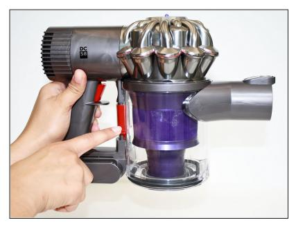
• Locate the red lever parallel to the red trigger and on the side of the clear bin.
