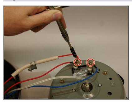
Remove red and blue wires from heating element to fully detach from control module. This is done by removing the screws on the heating element terminals using a Phillips head screwdriver, size PH2.
