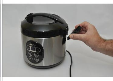
• Gently remove the piece that was held in place by the screw, you do this by pulling out from the top, then pulling up. This will expose the hinges for the lid.
