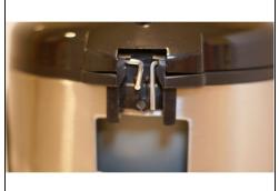
• To remove the hinge, gently rotate the bottom of the rod upwards, then push inward to pull the rod out. Repeat the process for each rod. This will allow the lid to be removed.
