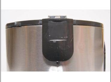
• Locate the piece on the black plastic trim that is opposite from where the hinges were. Carefully, pry this piece from the bottom to get the tab from behind the stainless steel to in front of the steel as shown.
