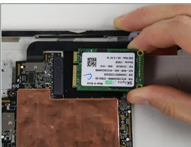
Lift up and pull gently on the SSD to remove it from the black connector.
