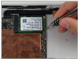
Remove the two 4 mm T3 Torx screws securing the SSD.
