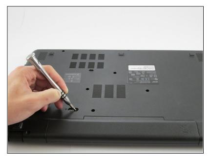
Place the pointed end of a spudger into the battery lock.
