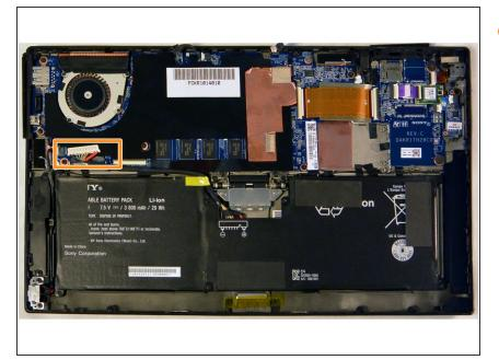
Disconnect the battery from the motherboard by pulling out the cable below the fan.
