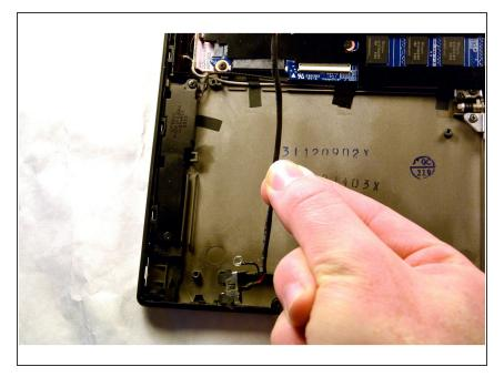
• Pull out the cable and jack assembly.
