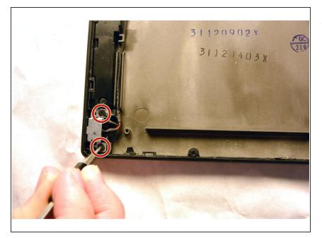
Remove the two 3mm Phillips #000 screws from the bottom left corner of the device.
