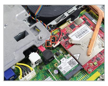
Disconnect these two power connectors on the motherboard, one connector is white and the other is black. You can identify the correct wires by their braided colors: red, yellow, blue, and black.
