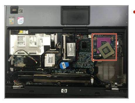
Lift up the processor carefully to remove
