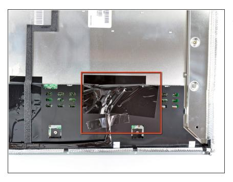
Remove the large piece of tape covering the inverter cable connector and any tape securing the cable to the inverter board.
