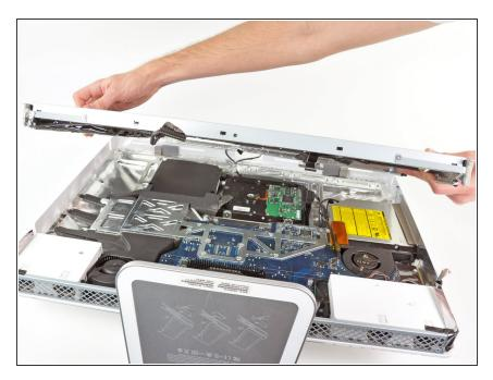
Remove the display assembly from the iMac.
