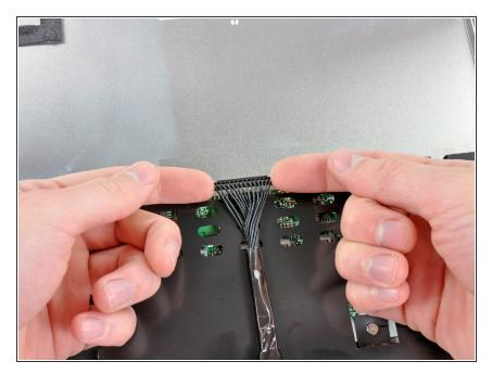
Lift the inverter cable connector straight up from its socket on the inverter board.
