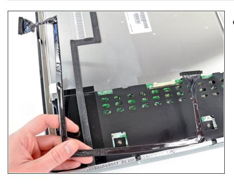
Remove the inverter cable from the LCD.
