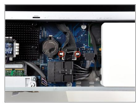
Remove the two T6 Torx screws securing the display data cable to the logic board.
