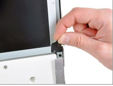
Peel the two highlighted EMI shield tabs off the frame of the LCD.
