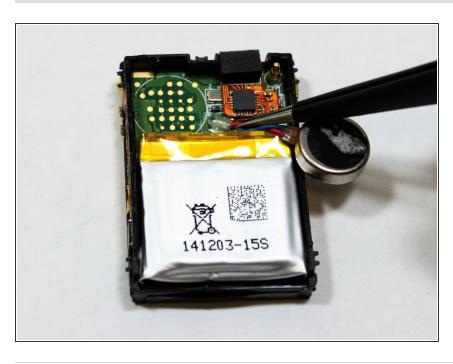
Use a pair of tweezers to detach both the blue and red wires from the motherboard.
