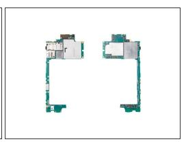
Release connectors on the motherboard. Remove motherboard.
