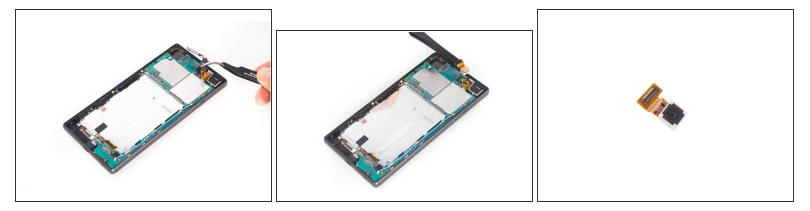
Remove that securing bracket, then remove front camera.
