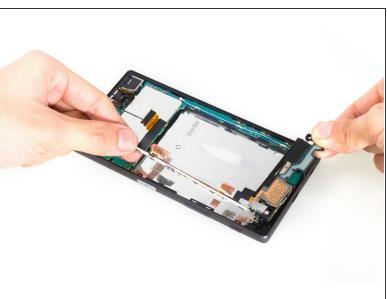
Remove main flex. (Attention: the fingerprint sensor connector is here, be careful to loosen it)
