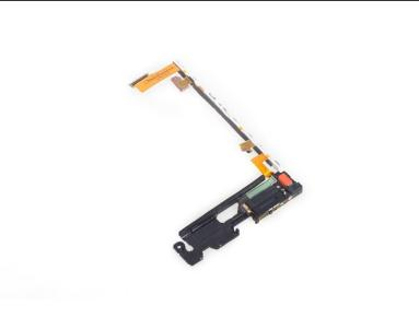
This is main flex assembly. (It comes with loudspeaker and vibration motor)
