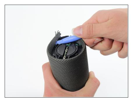
• Use a plastic opening tool to pry the sleeve off from the bottom of the speaker.
