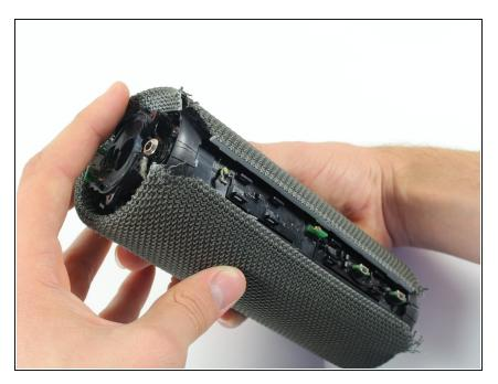
• With the switch plate disconnected, remove it and your device should now look like this.
