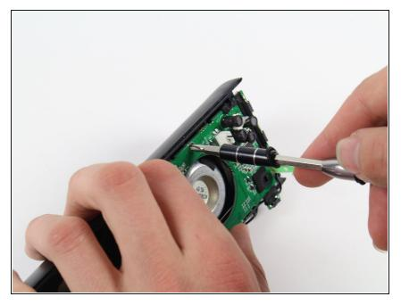
• With the Phillips #2 screwdriver, unscrew the 9.9 mm screw from the larger circuit board surrounding the speaker.
