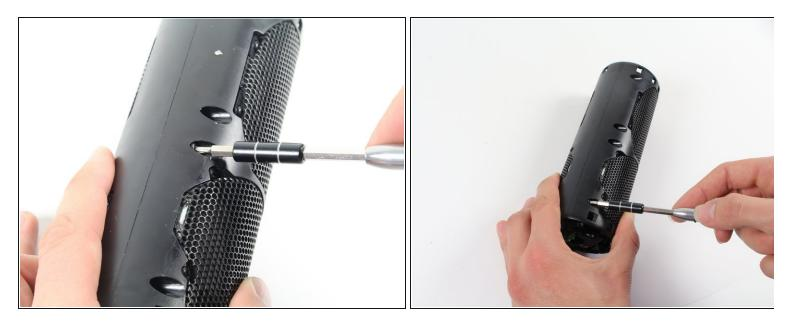
• Use a Phillips 1 screwdriver to unscrew the eight black 14 mm screws along the length of the casing.
