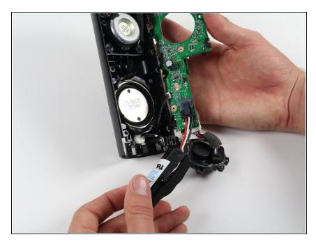
• Once all of the screws are gone, you should be able to remove the circuit boards and find the battery.
