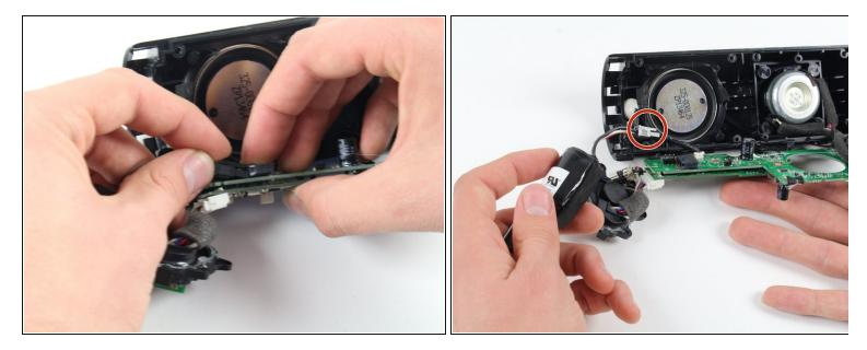
• Remove the battery by pulling it from the terminal as marked in the picture.
