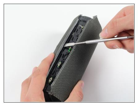
• With a metal spudger, pry open the tabs on the speaker sleeve along the length of the speaker.
