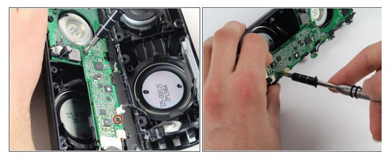
With a Phillips #00 screwdriver, unscrew two 5.6 mm screws from the rectangular shaped circuit board.
