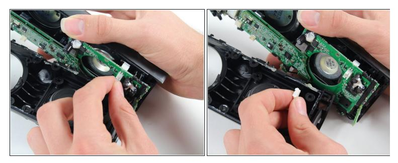
• Remove the speaker by pulling it from the terminal as marked in the picture.
