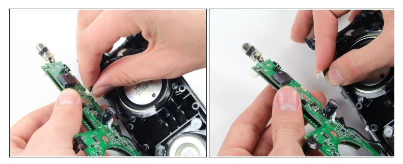
• Finally, remove the motherboard completely by pulling it from the terminal as marked in the picture.
