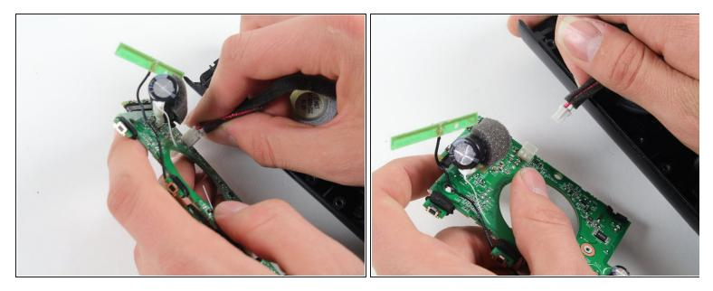
• Remove the second speaker by pulling it from the terminal as marked in the picture.
