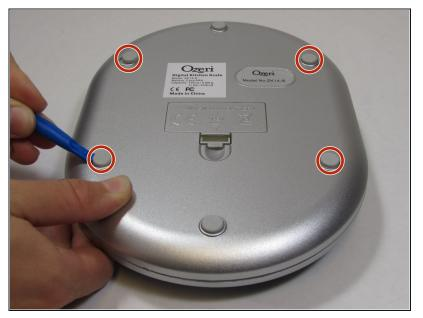
Using the iFixit opening tool, pry off the two rubber stubs on the right side and the two rubber stubs on the left side of the bottom of the device.
