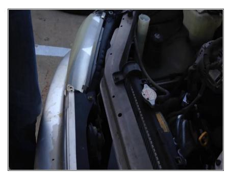
Locate the headlight bulb plug (right side headlight plug shown). This can be found underneath the hood and is positioned directly behind the headlight.
