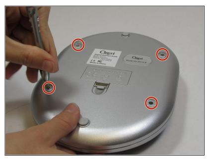
Using a 2.0 Flathead screwdriver, remove the four 9.46 mm Phillips head screws that were under the rubber stubs.
