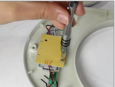
• Using the <u>2.0 Flathead</u> screwdriver, remove the three 7.20 mm screws on the back of the center LCD motherboard.
