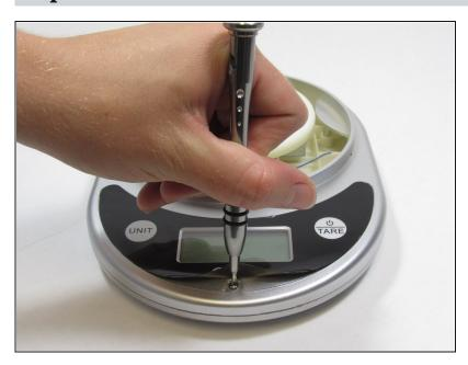
Using a 2.0 Flathead screwdriver, remove the 9.50 mm Phillips head screw under the sticker.
