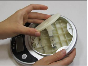
• Using a 2.0 Flathead screwdriver, remove the two 18.76 mm Phillips head screws in the plate stand.
