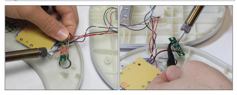
• Desolder the four posts in the center of the motherboard.
