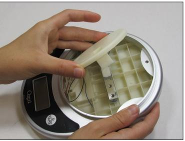
• Using a 2.0 Flathead screwdriver, remove the two 18.76 mm Phillips head screws in the plate stand.
