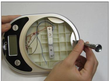
• Using a 2.0 Flathead screwdriver, remove the 9.44 mm Phillips head screw on the edge opposite to the LCD screen.
