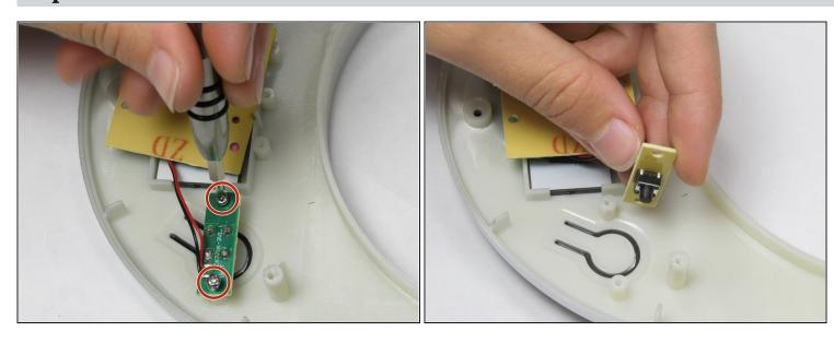
• Using a <u>2.0 Flathead</u> screwdriver, remove the two 7.34 mm screws on the smaller motherboards.
