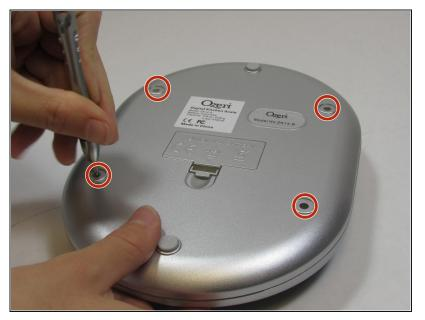
Using a 2.0 Flathead screwdriver, remove the four 9.46 mm Phillips head screws that were under the rubber stubs.
