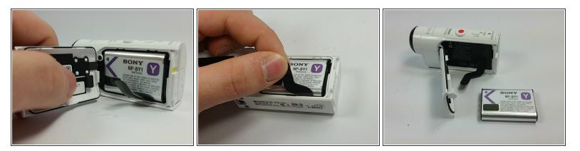
• Open the side panel outward to reveal the battery.
