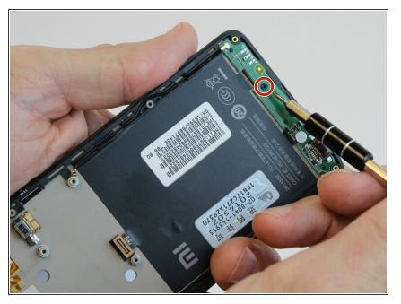
Remove the 2.9 mm Phillips #000 screw that holds the PCB circuit board to the screen assembly.
