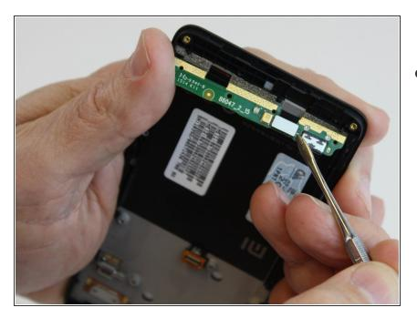
Using the nylon or metal spudger, pry back the silver clip covering the ribbon connector.
