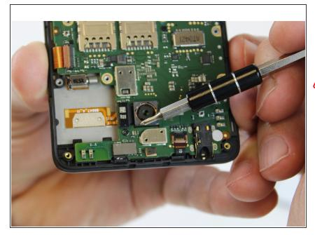
Remove the 3.4 mm Phillips #000 screw that holds the motherboard to the front body.
