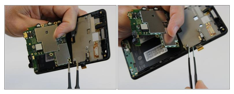
• Using the tweezers, pull the antenna connector from the motherboard.
