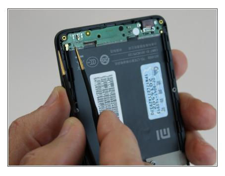
Using the tweezers, lift the antenna connector from the PCB circuit board.
