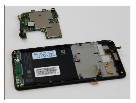
• Lift the motherboard out of the front cover and set aside.
