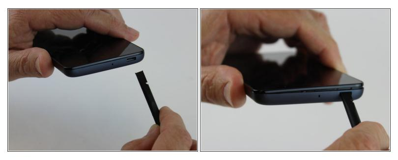
• Use the flat end of the spudger to remove the back panel from the mid-frame and front body.
