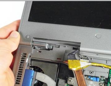
Lift the display module directly upwards from the base of the computer.
