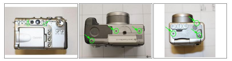
• Step 1. Remove: Remove the indicated screws from the camera.
