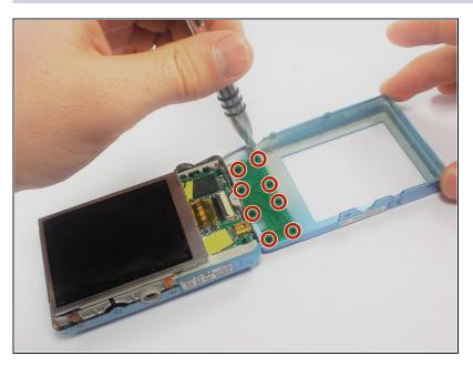
Remove the eight black screws connecting the keypad circuit board to the rear panel.
