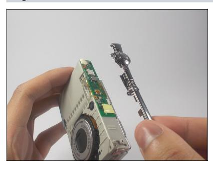
Gently remove the loosened chrome frame and connected shutter button from the camera.
