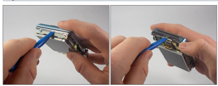
• With a plastic opening tool, gently remove the chrome framing on the left and right sides of the camera.
