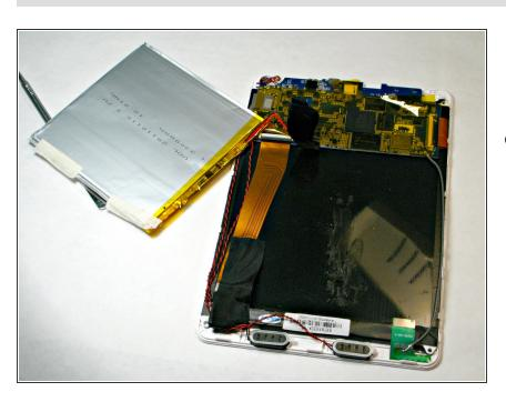
The battery is now disconnected from the tablet and can replaced. Re-installation of the new battery and tablet assembly can be completed by following the same steps in reverse. To reassemble your device, follow these instructions in reverse order.
