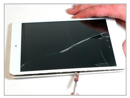
Starting near the middle edge of the Trio Stealth-G4X tablet, gently work the pry tool in between the seams of one side of the tablet.
