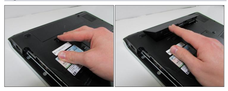
Slide the tab all the way over to the left until battery pops out. Lift out and remove battery.
