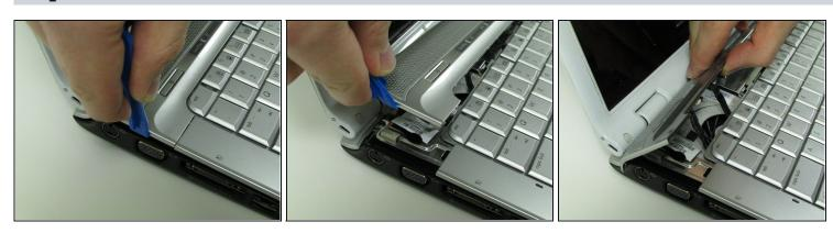
• Use an iFixit opening tool to pry open the plastic bar above the keyboard.
