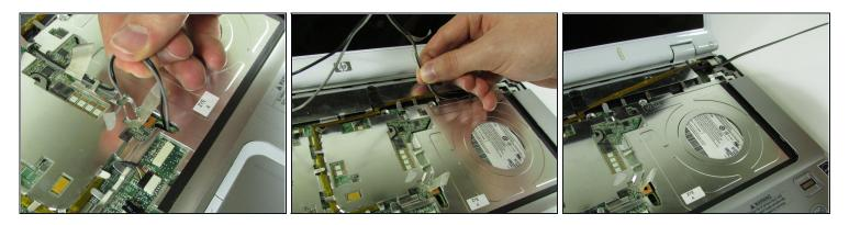
• Pull up on the WiFi wires and out from under the metal tabs.
