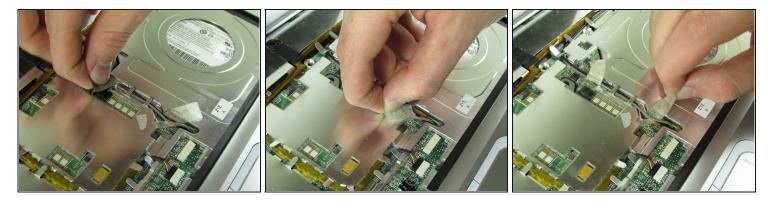
• Pull up on tape holding down wires.
