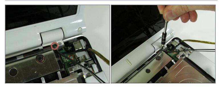
• Use a Phillips #00 screwdriver to remove the black screw located in the top right corner near the display.
