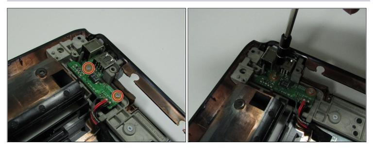
• Remove the screws securing the charging port.
