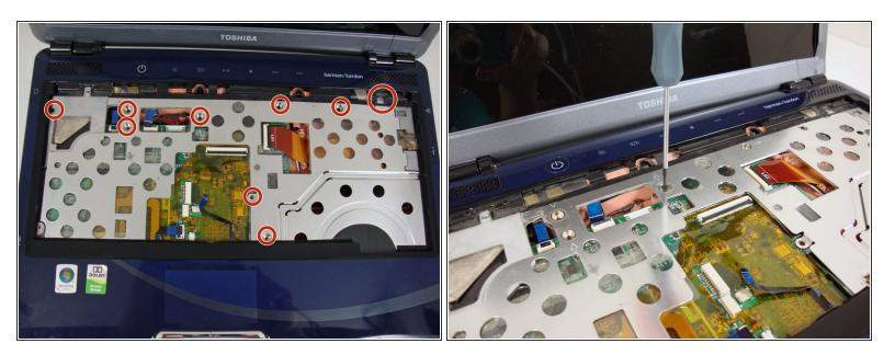
Remove the circled screws with Phillips #0 screwdriver.
