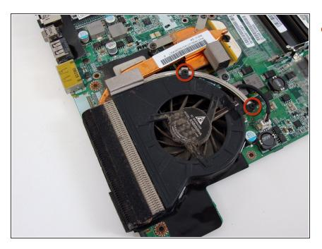
Remove the circled screws with a Phillips #0 screwdriver.
