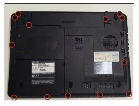
Remove these screws from the underside of the laptop with Phillips #0 screwdriver.
