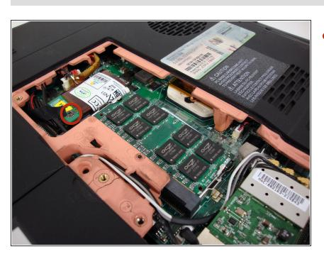
Remove the circled screw with a Phillips #0 screwdriver.
