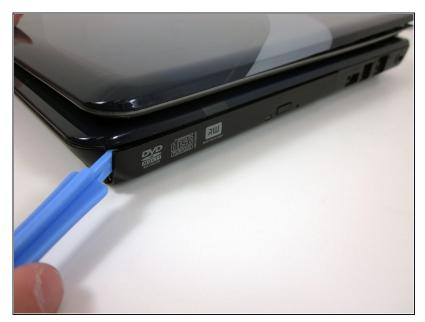
Use the plastic opening tool to pry the CD/DVD drive out of the frame.
