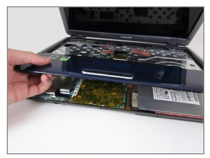
Remove the top plastic cover by lifting upward from the bottom left-hand corner as shown. The cover will come off easily.
