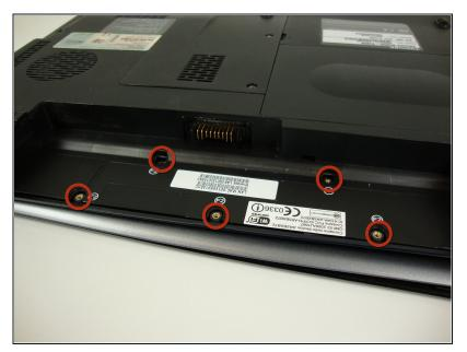
Remove the five "F2" screws with a Phillips #0 screwdriver.
