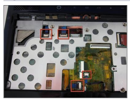
Detach the four blue ribbon cables carefully with tweezers.
