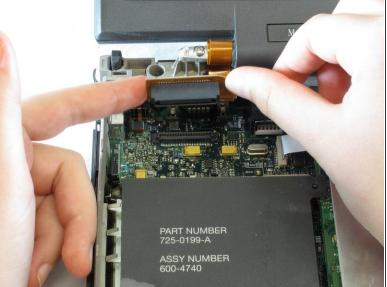
Gently pull up on the ribbon cable connection that connects the screen to the logic board.
