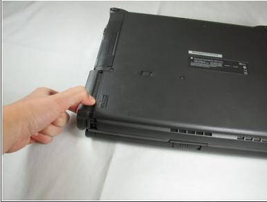
Hold the button on the front left side and slide the battery out.
