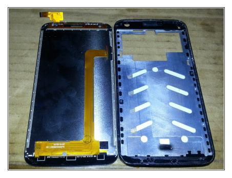
You should now be about to replace the screen with another one. The glass + Screen + Digitiser are all fussed together. This means all three part will need to be replaced if one of them fails. This is becoming the norm with most mobile today.
