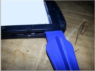
Using a plastic prying tool to carefully separate the back plastic cover (first mid frame) from the second mid frame. I recommend starting at the bottom and slowly work your prying tool around from there.
