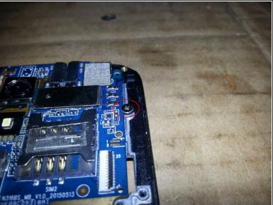
The main board is held in by one pillips head 1.8 x 40mm screw. I have marked this screw in red on the picture.
