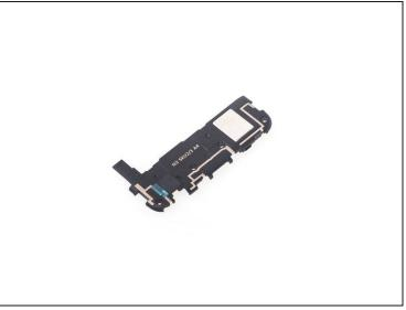
• A flexible clip is here. Loosen it and get the loudspeaker assembly only.
