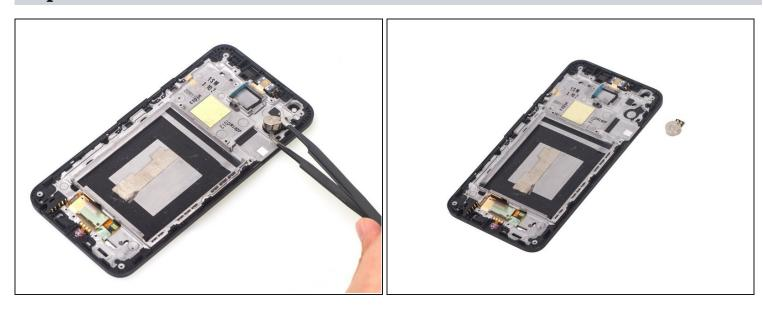
• Adhesive underneath vibration motor is a little bit strong. Pry it up carefully.
