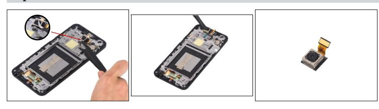
• The adhesive underneath rear camera is strong. Be careful to pry up and remove it.
