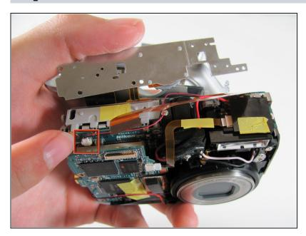
Carefully pull out the plug connecting the LCD to the motherboard.
