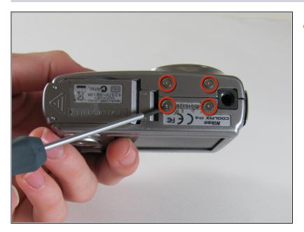
Remove the four 2.2 mm screws located on the bottom of the camera.
