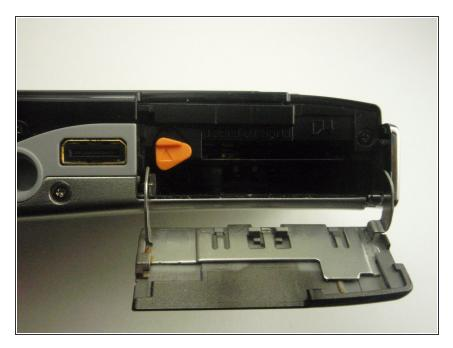
Push memory card further into the camera. This will release the memory card making it available to remove.
