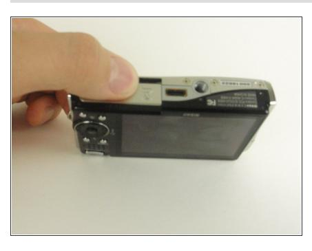
Slide the battery door in the direction of the arrow, toward the LCD screen. The door will then swing open.
