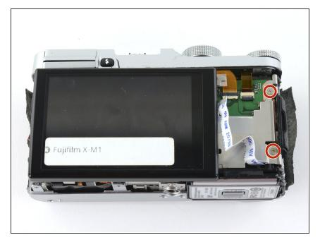
Remove the two 2.6 mm Phillips screws from the right side of the metal frame.
