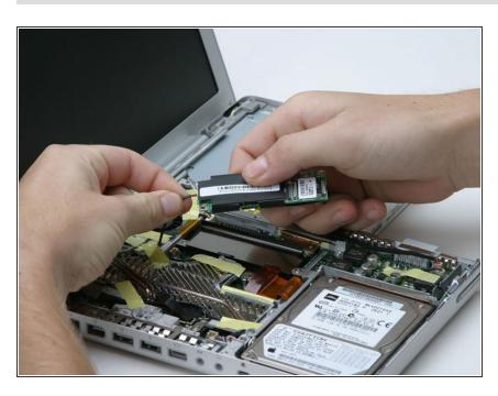
Disconnect the modem cable from the modem.
