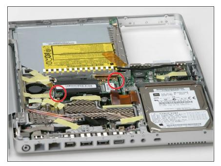
Remove the two Phillips screws from the corners of the modem.
